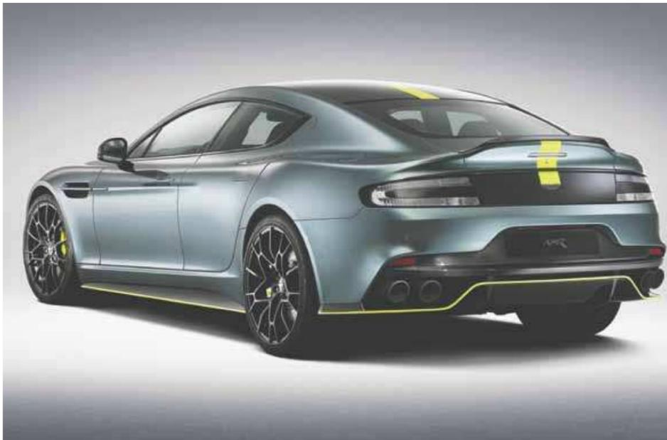
lift while retaining a neutral balance and the extra aerodynamic bodywork such as the splitter, sills, rear diffuser and boot lid lip spoiler are all carbon fibre. The new bonnet with large ventilation inserts is also made from carbon fibre to minimise weight.
