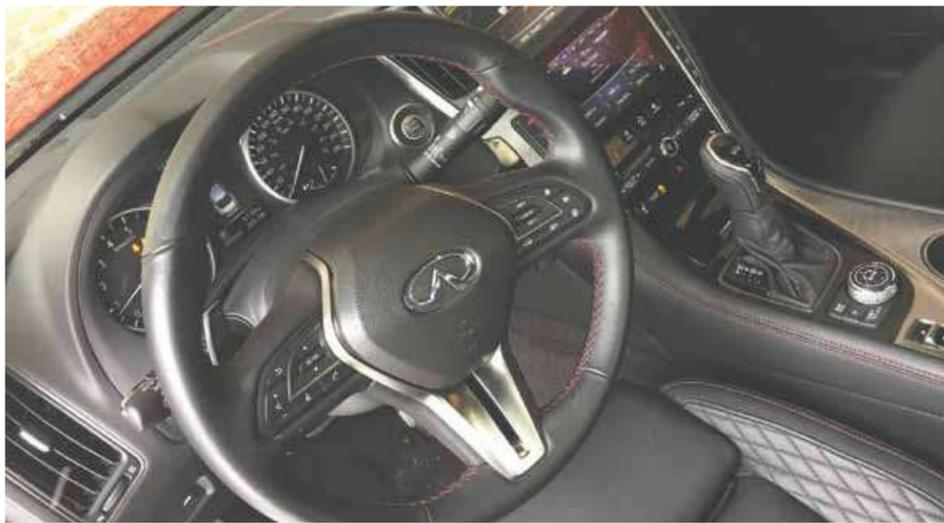
ogy. The Q50 was the world’s first production car to feature a steer-by-wire system, which means, that the steering wheel is not mechanically connected to the front wheels, so your steering
